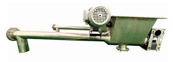
Micro-Feed Screws are auxiliary screws combined with a larger main screw feeder. Before reaching the set feed rate the main screw feeder is stopped by a proximity switch to allow the Micro-Feed Screw, which is flanged beneath an opening in the pre-outlet section of the main screw feeder pipe, to feed the missing quantity of material with high accuracy through the outlet of the main screw feeder-into the weigh hopper.
